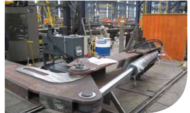
Actuator arm prior to installation
